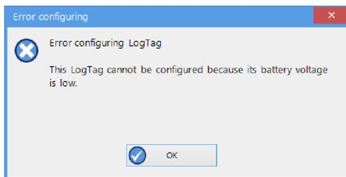
If your logger has a user-replaceable battery, it needs to be changed now. Loggers without replaceable batteries need to be discarded and replaced.
