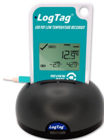
Figure 4: Logger used with interface cradle
