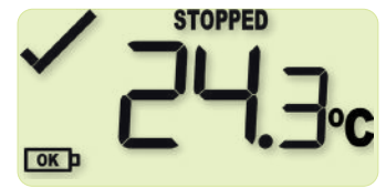
Figure 19: HAXO-16BT display while the user is pressing the START button, REC• disappeared
