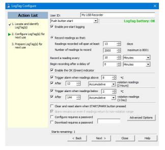
Figure 1: USRIC-8(M) Standard Configuration Options
