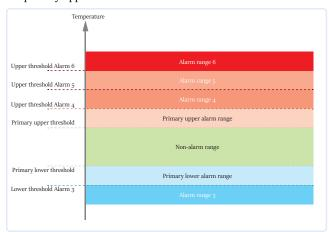
Figure 3: Alarm ranges and thresholds example
