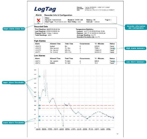
Figure 6: Sample report page with Multiple Alarm Thresholds
