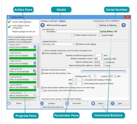
Figure 37: Configuration screen for a HAXO-8
