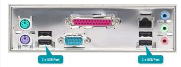
Figure 34: Rear of PC with 4 USB ports
