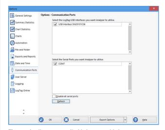
Figure 148: All COM ports disabled, USB enabled
